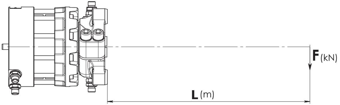
Load diagram for rotator GR55FF
